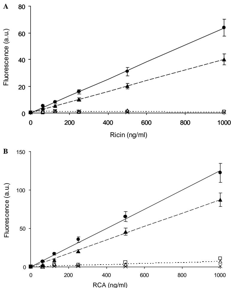
Fig. 6. Binding specificity of ricin (A) and RCA (B) with microchip-immobilized saccharides: lactose (●), disaccharide B (▲), A<sub>tri</sub> (△), B<sub>tri</sub> (□), and mannose (x) (2.5 mg/ml gel).
