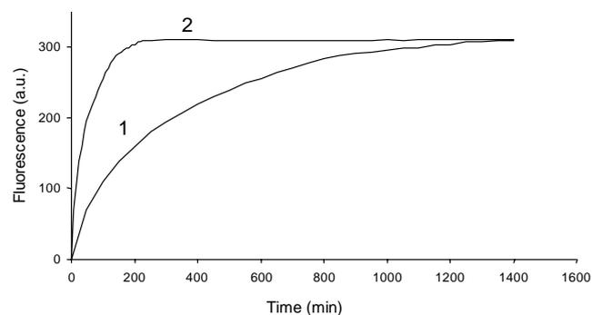
Fig. 4. Kinetic curves for binding of ricin with chip-immobilized lactose obtained without mixing (1) and with mixing with peristaltic pump (2). Concentration of ricin-Cy3 in solution was  $1.5 \times 10^{-9}$  M, concentration of immobilized lactose was 6.5 pmol/gel element.
